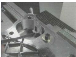
On Lower Rocker Box - Relieve Area Around Valve Spring and Note That Bolt Boss Has Been Relieved, as well, to Clearance Top Spring Collar
